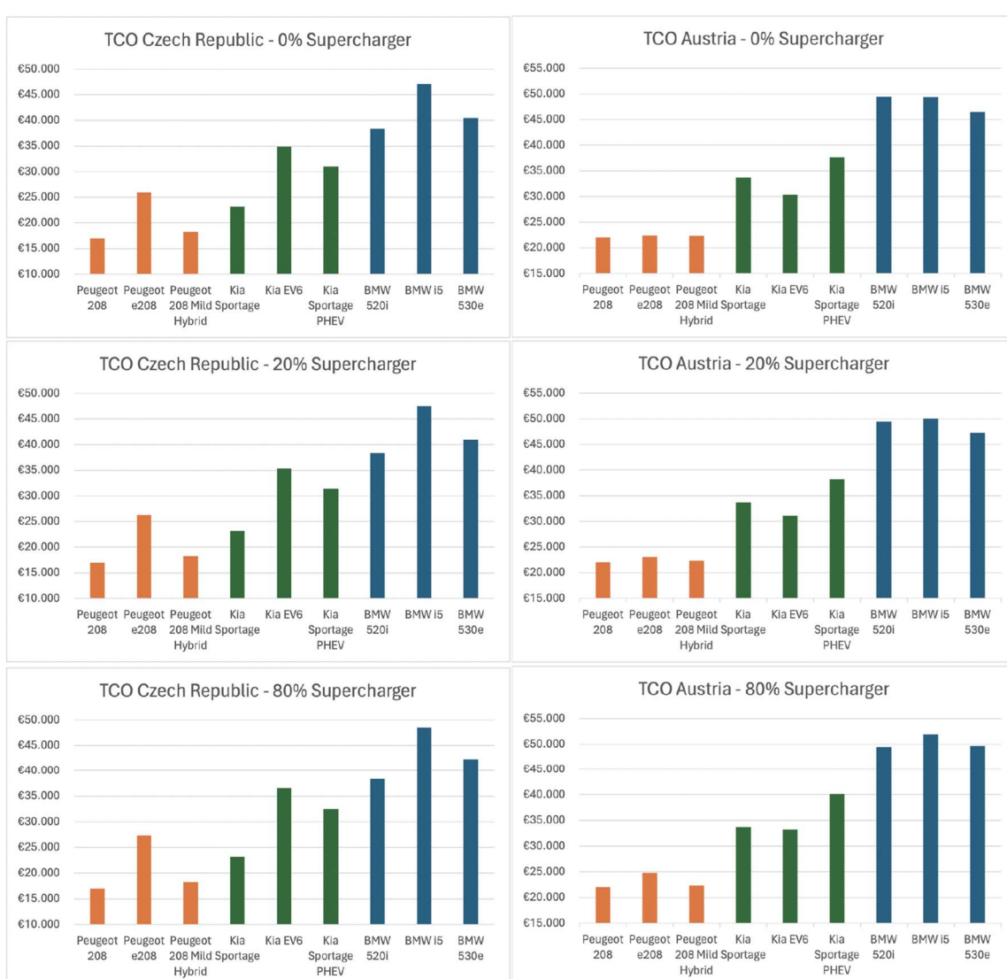
Results of TCO calculations with different Supercharger usage: orange - subcompact segment; green - compact segment; blue - executive segment
